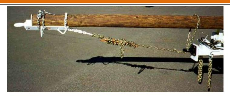
The PM-10 Pole Muzzle Continues to gain recognition in the utility industry as the best solution for pole hauling problems. Strong and rugged, the PM-10's simple design offers durability and ease of installation for many years. Designed to fit the lead pole, the PM-10 provides solid cinching to the pole and allows for chain binding back to the pole trailer for added safety during transportation. The PM-10 has a slotted back that allows for bolting through the gain hold for added security.
